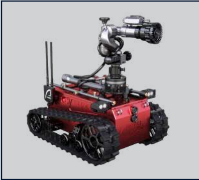
WATER / FOAM MONITOR
