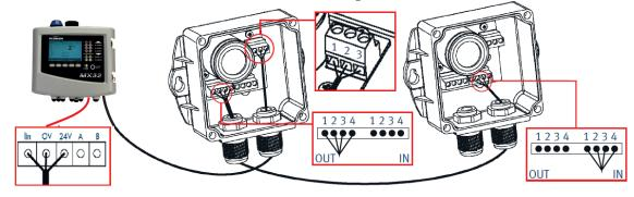
Wiring of 1 OLCT 10 SC (with a semi-conductor cell)
