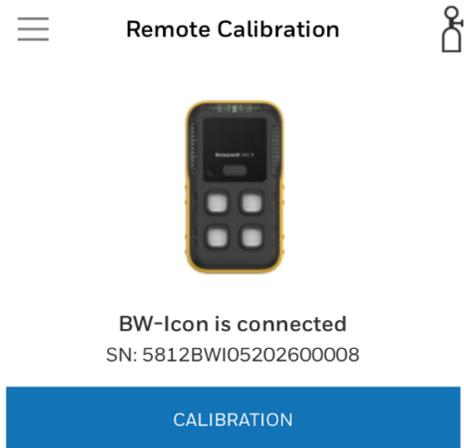
**Note:** If sensors fail to detect the gas, or cannot be spanned, repeat the calibration. If the problem persists, replace the sensor.
