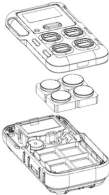
3. Remove the sensor filter from the inside of the front enclosure.
