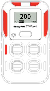
A Honeywell BW Flex-i handheld device with a monochrome screen displaying '200 HIGH'. The screen also shows 'H2S 0.00' and 'Honeywell BW Flex-i'. The device has a keypad and a speaker. | "HIGH" message is displayed. Alarm LEDs alternately flash. Alarmed sensor LED flashes too. It beeps and vibrates. |
