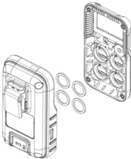
4. Place a new filter in place. Peel down the filter from the baseboard and stick it to the front shell.
