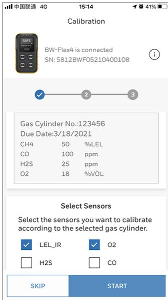
13. Open the cylinder valve by turning the pressure regulator knob counterclockwise. Follow onscreen instructions to know when to apply gas. The IntelliFlash lights amber.
