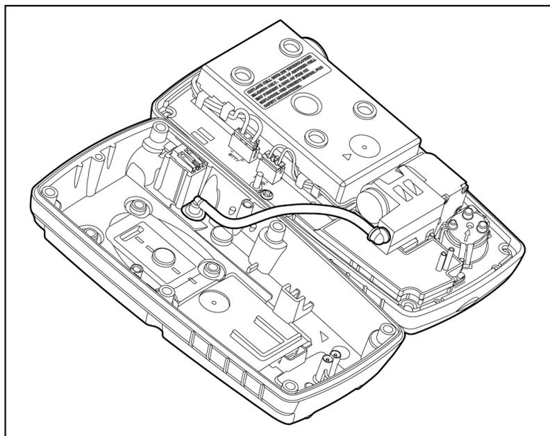
5. Remove the two PCB screws.
