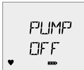
When the diffusion cover is replaced, the detector activates the pump alarm.
