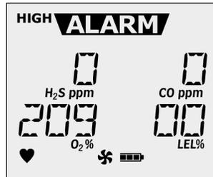
During a pump alarm, **HIGH** and **ALARM** display, and
