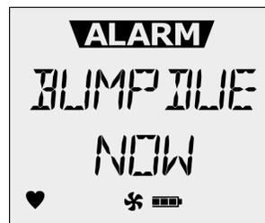
Apply gas while **BUMP DUE NOW** displays. Verify the visual, audible, and vibrator alarms activate. The detector must enter alarm to pass the bump test. For complete instructions, refer to See "Bump Test" on page 68 for more information..
