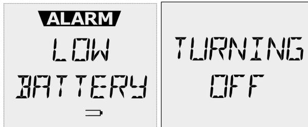
Recharge the battery for 6 hours and then reactivate the detector.
